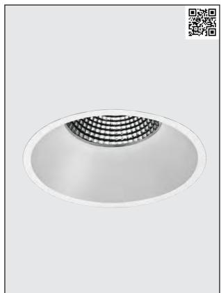
Compact LED Downlight with a deep reflector. Low glare (UGR <13). Glass standard included (IP44). Equipped with Philips Fortimo LED module and Philips Xitanium LED driver.
