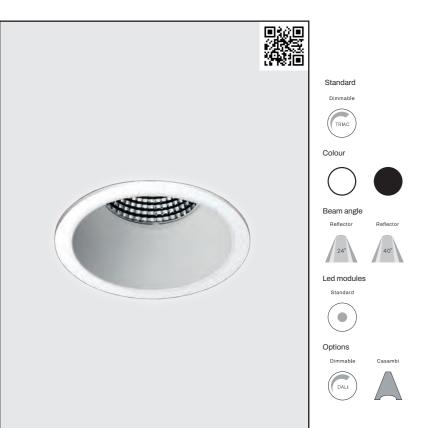
Fixed round recessed fixture with extra deep reflector and low glare. Standard Triac dimmable. Equipped with Philips Fortimo LED module and Philips Xitanium LED driver. IP44 set available upon request.
