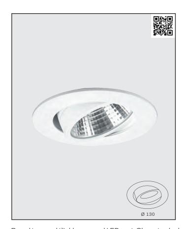
Round turn- and tiltable recessed LED spot. Glass standard included. Powder coating finish. Equipped with Philips Fortimo LED module and Philips Xitanium LED driver.
